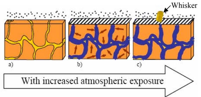
Figure 1. Model for whisker growth with the presence of a soft metal at grain boundaries of substrate material. a) oxygen interacts with material b) oxide layer forms at interface of SM and substrate grain, in addition to a thin native oxide layer at the surface (denoted by diagonal hatch marks), resulting in a compressive stress. c) compressive stress forces SM to yield and whisker forms.
