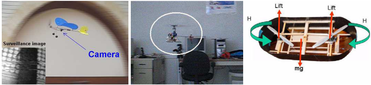
Figure 2: With a 18 inch wingspan, our fixed-wing aerial platform (left) can fly as slow as 2 m/s and carry a payload of 20 grams . Rotorcraft, such as helicopters (middle) and ducted fan engines (right), are difficult to fly.
