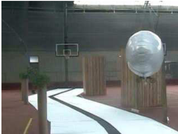
Figure 9: Swarthmore College’s blimp following the collision-free path.
