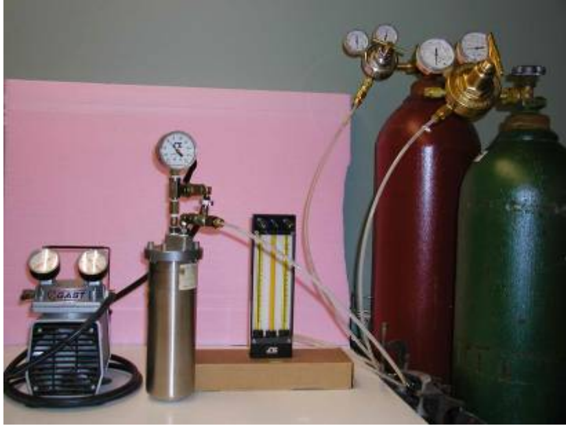
Figure 2.4 Low pressure cells: pressurization system
