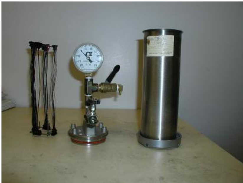
Figure 2.5 Low pressure cells: incubated samples with fix frames
